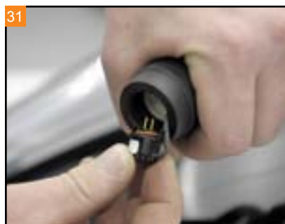
Plug the twist-grip sensor into the grip.
