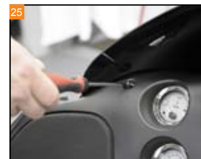
25 Install the six fairing mounting bolts.
