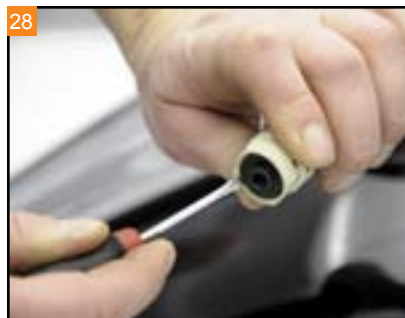
Pry the plug out of the twist-grip sensor.
