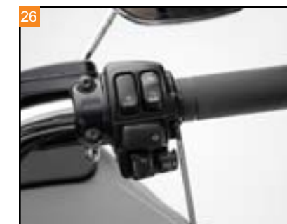
26 Remove the right-side switch housing hardware.
