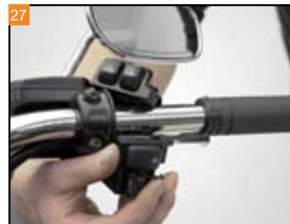
Remove the throttle grip.
