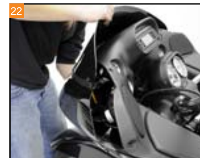
22 Install the outer fairing.
