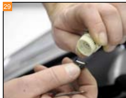
Removing the plug allows the sensor to be plugged into the heated throttle grip.
