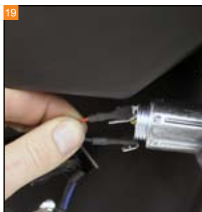
19 Plug the grip wiring into the cigarette lighter.
