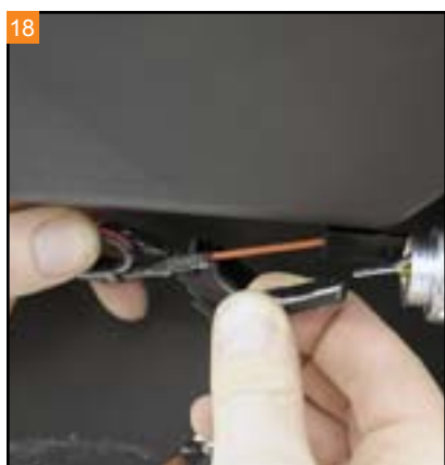
18 Remove the wiring to the cigarette lighter.
