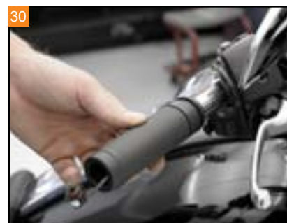
Slide the heated grip onto the handlebar.
