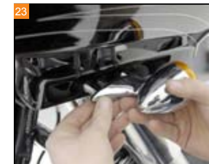
23 Install the turn signal mounting brackets.
