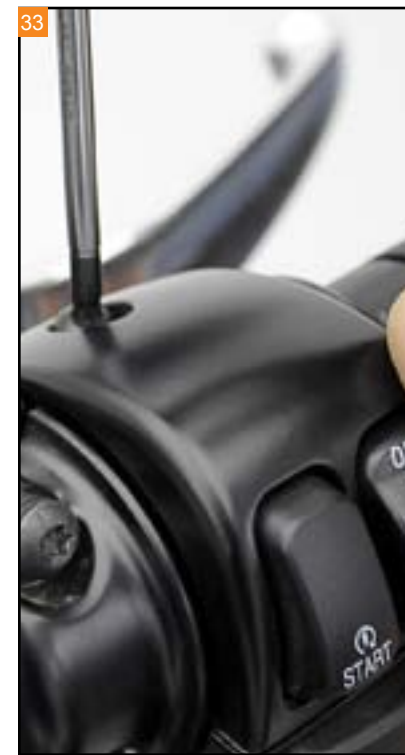
Tighten the switch housing mounting hardware.
