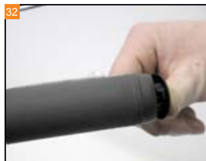
Install the end cap on the throttle grip.
