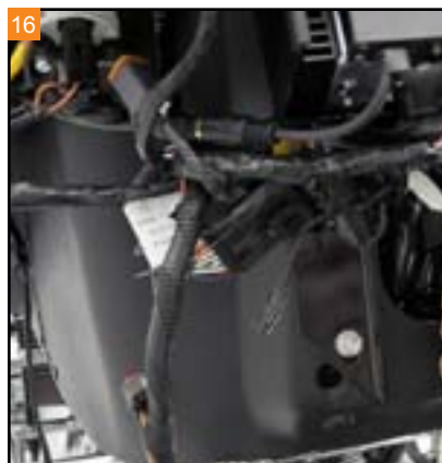
16 Pull the wiring through the inner fairing.
