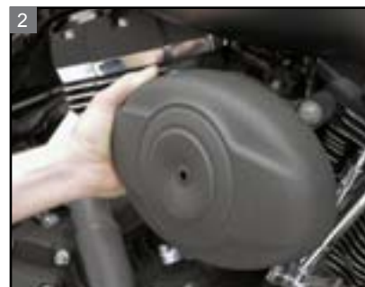
2 Remove the air cleaner cover.
