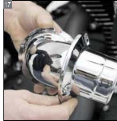
Slide the mounting ring onto the intake tube.
