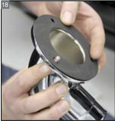
Install the intake tube gasket.
