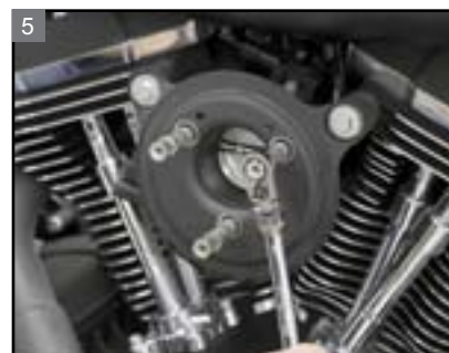
5 Loosen the back plate hardware.
