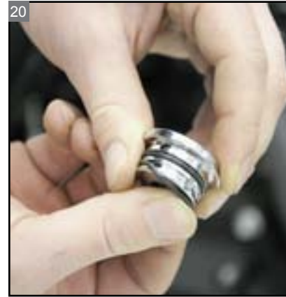
Install the sealing O-rings onto the breather plugs.
