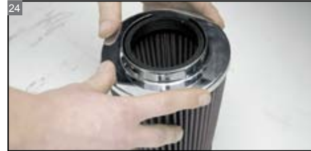
Stick the band clamp cover onto the filter element.
