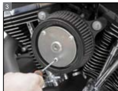
3 Loosen and remove the filter element mounting hardware.
