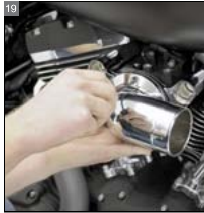
Install the intake tube mounting hardware.
