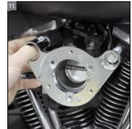
11 Loosely install the breather bolts.
