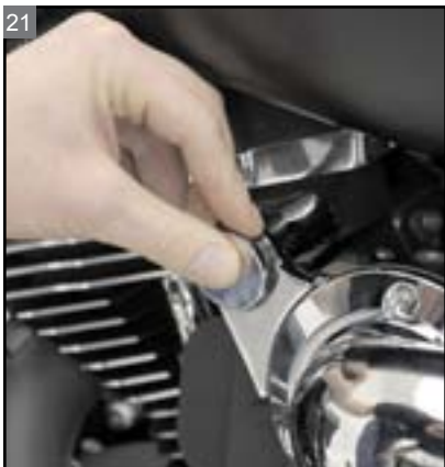
Push the plugs into the back plate.
