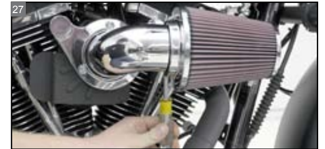
Tighten the band clamp.
