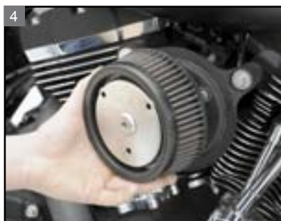
4 Remove the filter element.
