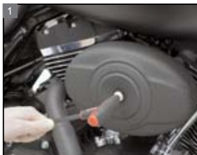
1 Loosen and remove the air cleaner cover mounting hardware.
