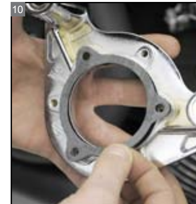
10 Stick the breather gasket onto the back plate.
