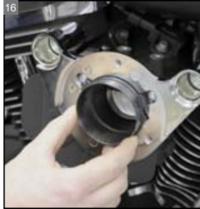
Install the adapter into the back plate.
