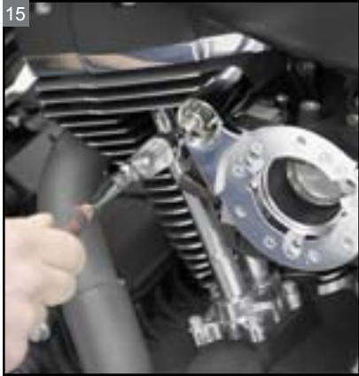
Tighten the breather bolts.
