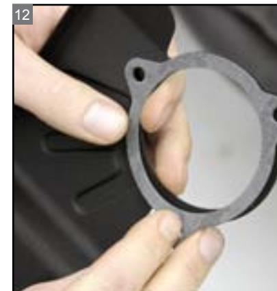
12 Install an intake gasket onto the throttle body cover.
