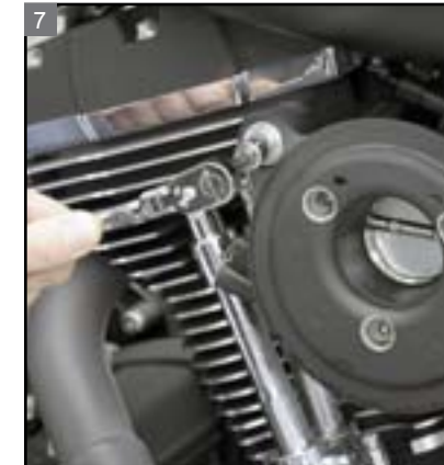
7 Loosen and remove the breather bolts.
