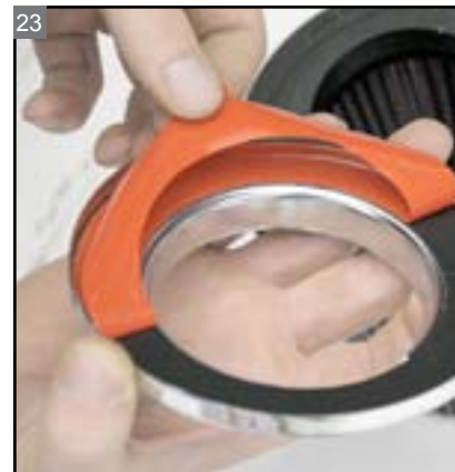
Peel the backing off of the adhesive ring.
