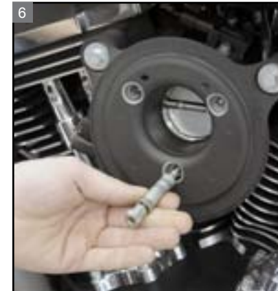
6 Remove the filter stand-offs.
