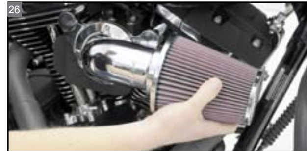
Install the filter onto the intake tube.
