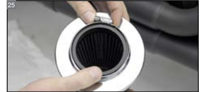
Install the band clamp onto the filter.
