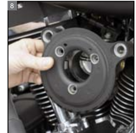
8 Remove the back plate.
